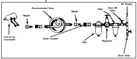
trigger on the tool. Disconnect the air line and pour into the intake bushing a teaspoonful (5ml) of a suitable pneumatic motor lubricating oil preferably incorporating a rust inhibitor. Reconnect tool to air supply and run tool slowly for a few seconds to allow air to circulate the oil. If tool is used frequently lubricate on daily basis and if tool starts to slow or lose power.
